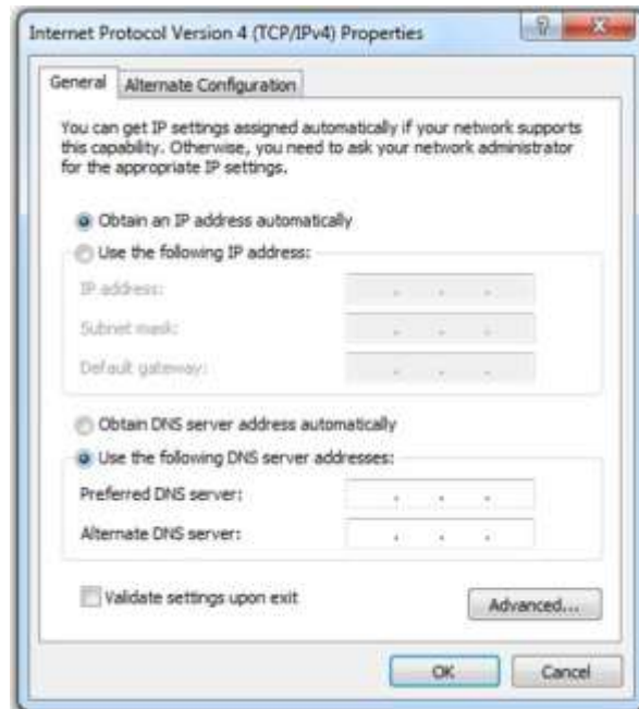
Figure 2-5 Windows Network Connections IPv4 properties page - DHCP
