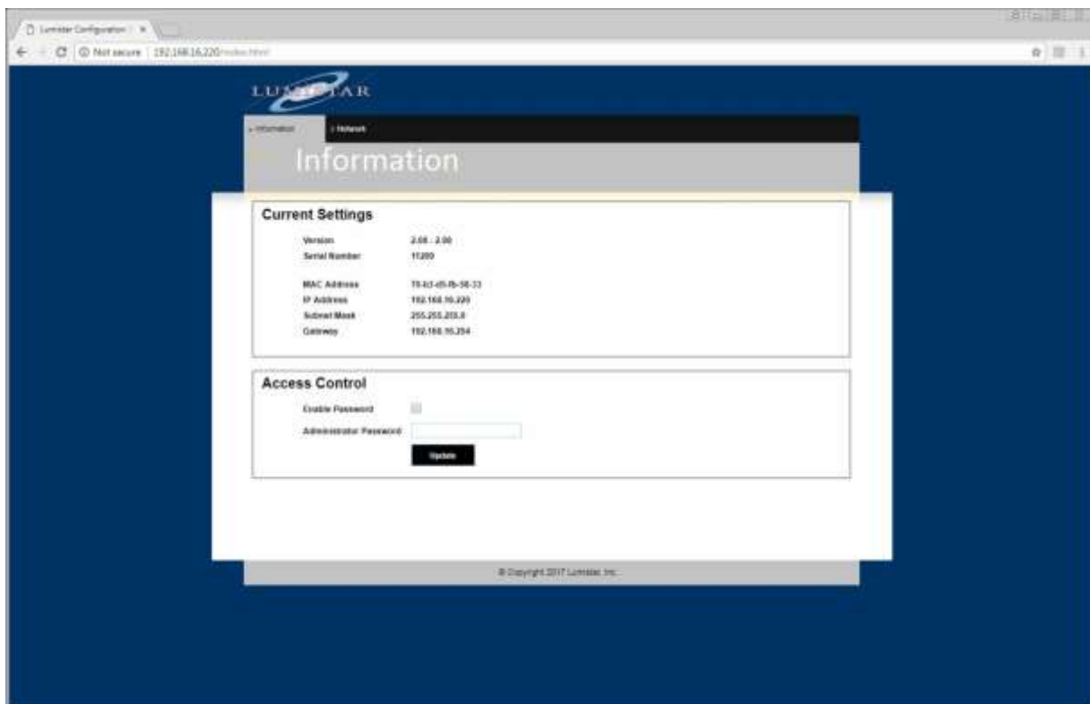
Figure 2-6 LS-28-DRSM Network Setup: Web Browser Information Setup Tab
