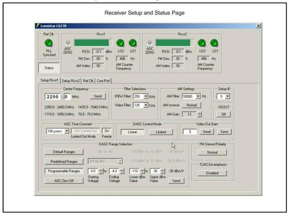
The figure above illustrates one of the two receiver control tabs as well as the status window for both independent receivers. Status is provided in the upper third of the GUI window. Status is provided for the following items:
