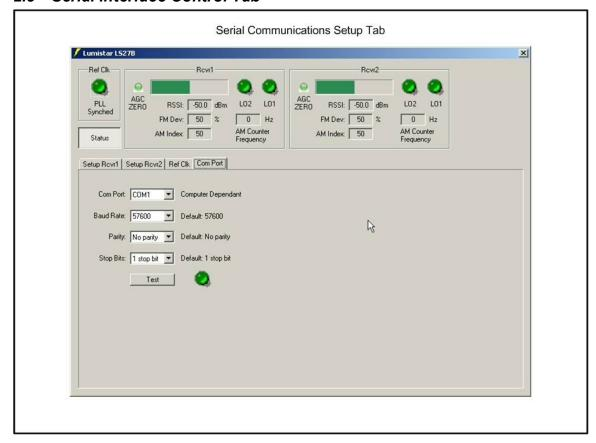
The figure above illustrates the serial interface control tab. From this tab the user can select from various host computer serial ports detected and set BAUD rates and communications formats. The unit's defaults are shown and should be used in normal operating conditions. Custom setups are possible. Consult the factory for details.
