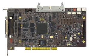
The IRIG Time Code Reader and Generator operate with IRIG A, B, or G time codes. The Time Code Reader is typically used to insert time information into the PCM minor frame block of data. The Time Code Generator creates and outputs time information in accordance with the IRIG Time Code Standards. Both reader and generator are capable of operating at <sup>1</sup>/<sub>2</sub>, 1, and 2 times the normal rate.
