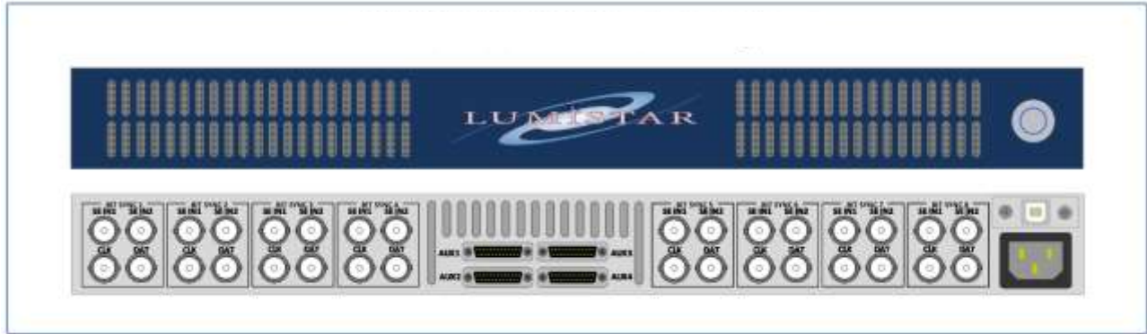
LS-45-R1-OBS Front and Rear Panel Elevations
