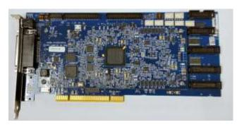
The Lumistar LS-45-P Dual Channel Bit Synchronizer Daughterboard provides optimal reconstruction of a serial PCM data stream that has been corrupted by noise, phase jitter, amplitude modulation, or base line
