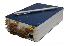
synchonization from external sources as well for Combined or Independent channel data from RF or IF. Digital multi-mode demodulation options include Multi-Symbol PCM/FM, SOQPSK, BPSK, QPSK, OQPSK, SQPSK, AQPSK, AUQPSK, PCM/PM, and Multi-H CPM. Sub-carrier(s) demodulation can also be provided, other formats available upon request.
