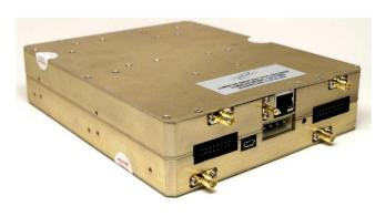
programmable AM/linear AGC outputs for auto-tracking receivers. The design offers 8 IF Bandwidths and 8 Video Filters per channel for each receiver. AC coupling with a low pass filter is employed to ensure a high quality data link with long strings of NRZ-L ones or zeroes. The unit provides a software selectable 10 MHz reference I/O port for locking local oscillators to a high precision external source or to arrange multiple units in a master/slave
