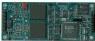
The Lumistar LS-40-DB25 Bit Synchronizer Daughterboards are used to provide optimal reconstruction of serial PCM data streams that have been corrupted by noise, phase jitter, amplitude modulation, or base line variations. The all-digital design assures a consistent product with high reliability and long-term stability. Please refer to the Lumistar LS-40-DB
