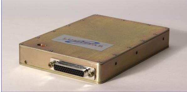
By packaging the LS-40-DB into the stand alone drive bay housing, the LS-40-B has the same Built-In Test features of both *Auto-Test* upon start up and *Command-Test* allowing the user to manually check the bit sync functions at any time. The bit synchronizer includes a data correlator for reading pseudo-random test patterns, as well as frame sync words. The user has the ability to generate internal pseudo-random patterns and
